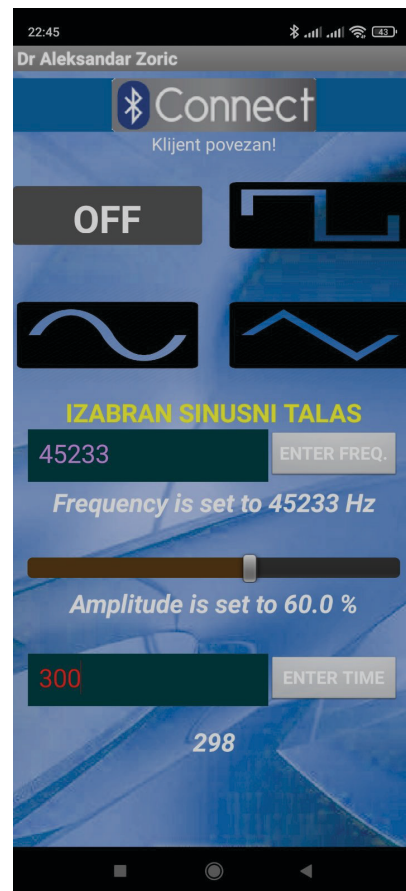
Fig. 4. The function generator application interface on a mobile phone
