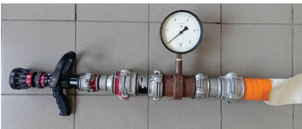
Fig. 1. Study changes in the geometric parameters of fire hoses when using the PROTEK 366 fire barrel.
