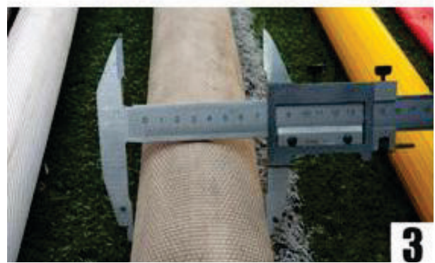
Fig. 2. Determination of the geometric parameters of the investigated fire hoses (change in diameter), 1 – pressure fire latex hose with a diameter of 51 mm, type T; 2 – pressure fire hose with double-sided polymer coating 51 mm, type T; 3 – pressure latex fire hose with a diameter of 77 mm, type T [1].
