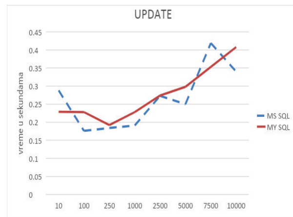
Figure 2: Results of measuring UPDATE records in the table (in seconds)
