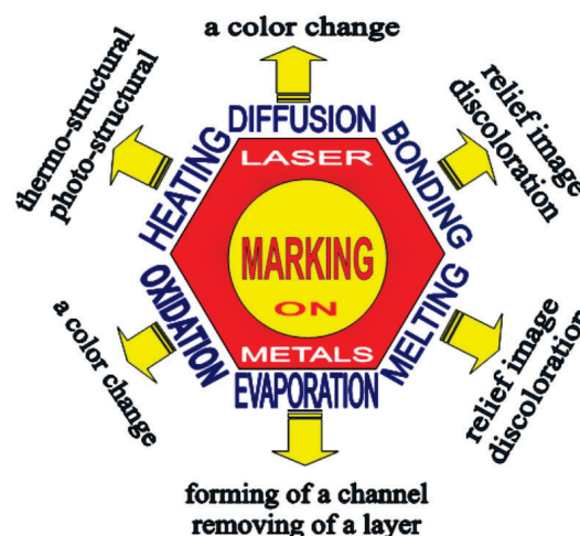
Fig. 1. Physical processes in laser marking on metals [2]
