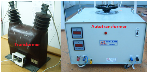
Fig. 1. The test transformer and autotransformer.
