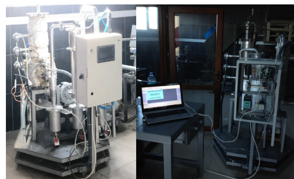
Fig. 3. General view of gasifier and control unit
