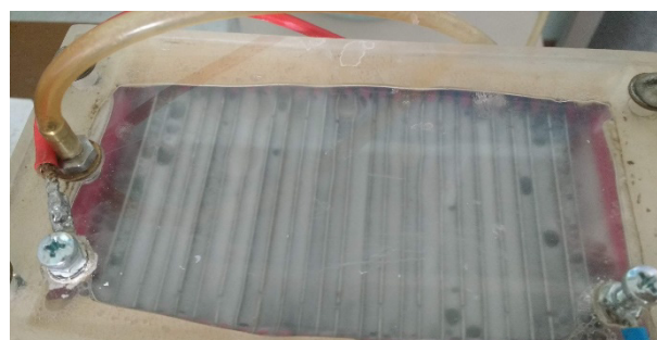
Fig. 3. Visualization of the electrolyzer operation. Gas emission is observed on all plates
