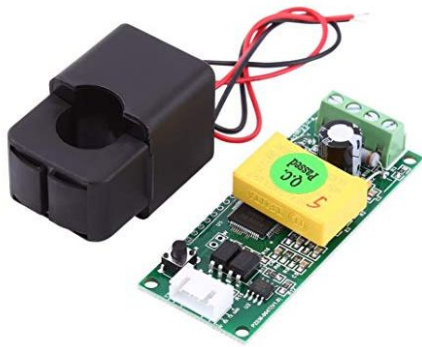
Fig. 2. PZEM004 module with a split current transformer as a current sensor.
