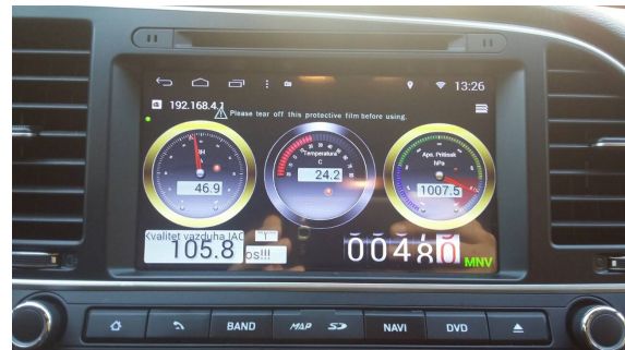
Fig. 5. Client Web page of the online weather station on a multimedia screen in a cabin of a car.
