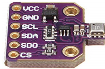
Fig. 2. CJMCU-680 module with BME680 sensor on the printed board.
