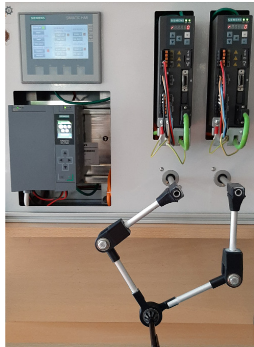
Fig. 4. Realized 2D delta robot
