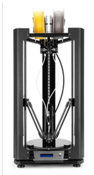
Fig. 3. 3D printer with parallel kinematics and linear actuators
