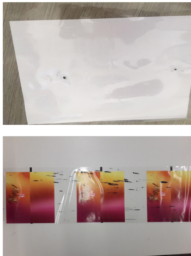
Fig. 1. Black dots and printing defects on package
