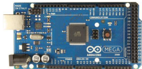
Fig. 1. Arduino Mega development card
