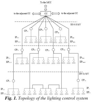
The use of the considered basic approaches in combination with the standardization of the elements of the control system allows the use of a hierarchical integrated principle of building a control system for city lighting systems, which provides the possibility of unifying elements and modifying its software. At the same time, the use of microprocessor and computer technology allows automating not only technological processes, but also the processes of processing and storing information.
