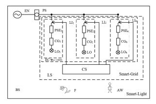
Fig. 3. Biotechnical lighting system. \* EN - electrical network, PS - power source, PSE - protective and switching equipment, control gear ~ starting and control equipment, LO - light sources, LI - lighting installations, EC electrical complex, CS - control system. LS lighting system, F - flora, AW - animal world, BS -
