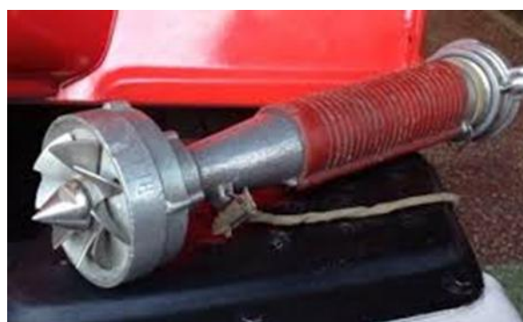
Fig. 1. Type of NRT-5 nozzle on the branch pipe RS-70 (main characteristics of the nozzle: working pressure - 0.4-0, MPa, water flow - 5 l/s, water jet supply range - 20 m, nozzle outlet diameter 7.5 mm)
