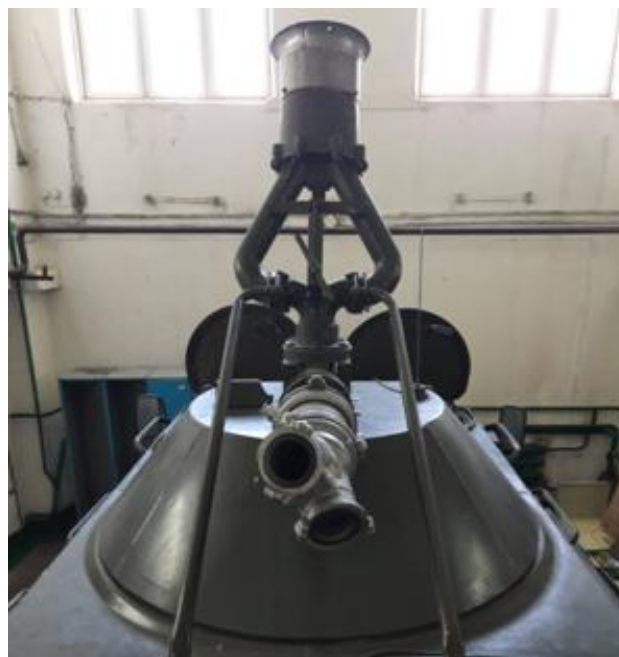
Fig. 3. View of the developed branch pipe installed on the armored personnel carrier BTR-60 PB (State Service of Emergencies of Ukraine in Nikolaev region, protection guard of the South-Ukrainian nuclear power plant)
