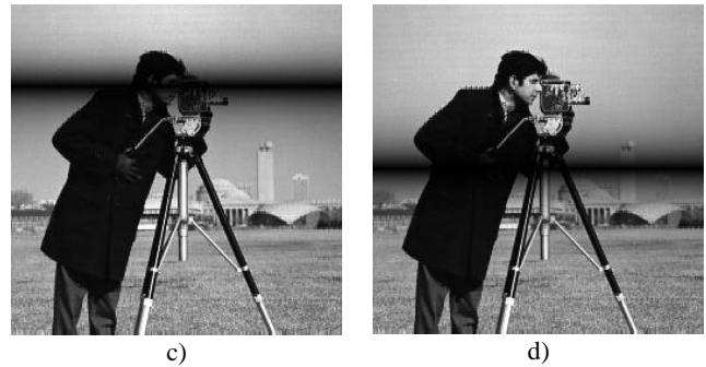
Fig. 4 Visual appearance of image after applying the Notch filter for: a) \omega_c = \pi / 4 and r = 0.9 , b) \omega_c = \pi / 2 and r = 0.9 , c) \omega_c = \pi / 4 and r = 0.5 and d) \omega_c = \pi / 2 and r = 0.5 .
