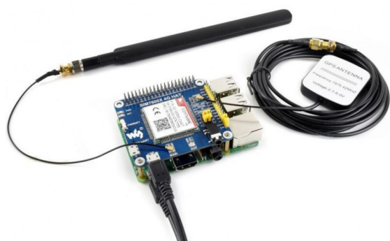
Figure 3. The SIM7600E-H-4G HAT mounted on the Raspberry Pi 3B+
